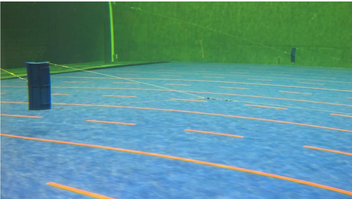
Flydeskovle testes i prøvetanken i Hirtshals.
